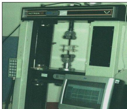
Fig 1 Transfer of specimen onto test plates mounted in Instron Universal Testing Machine using custom storage jig
